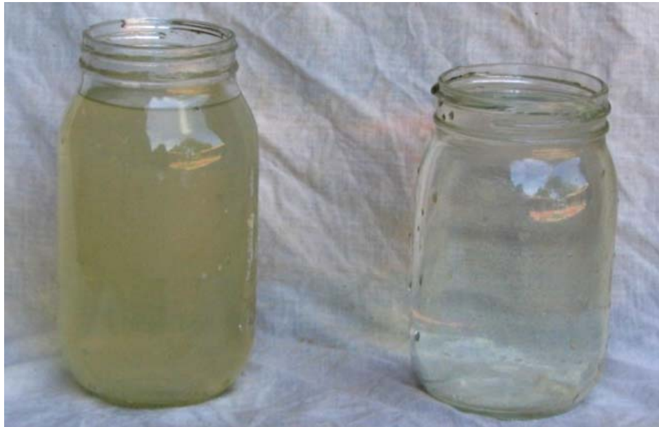
Figure 75: Effluent water sample (right) from HydrAid™ BioSand Filter Sibi 07 showing “Clear” color in comparison with the raw source water (left)
