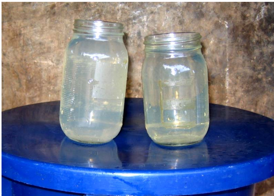
Figure 81: Effluent water sample (right) from HydrAid™ BioSand Filter Sibi 09 showing “No Apparent Changes” in color in comparison with the raw source water (left)
