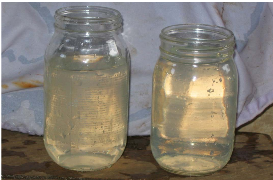
Figure 87: Effluent water sample (right) from HydrAid™ BioSand Filter Sibi 11 showing “No Apparent Change” in color in comparison with the raw source water (left)
