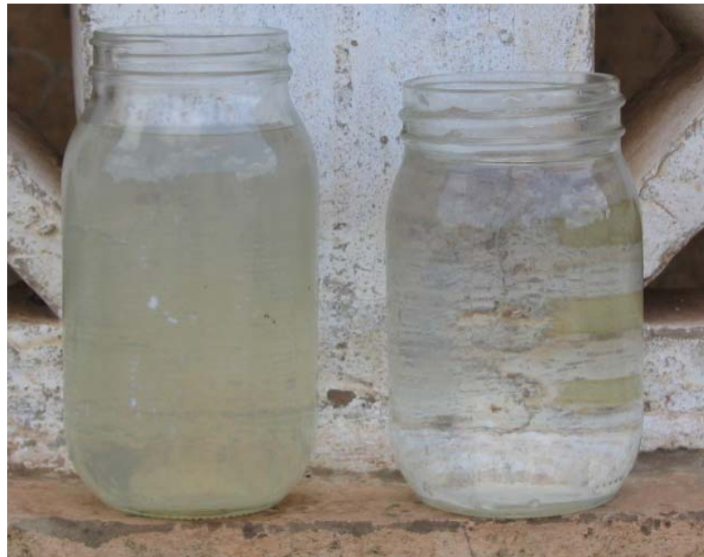
Figure 66: Effluent water sample (right) from HydrAid™ BioSand Filter Sibi 02 showing “Very Clear” color in comparison with the raw source water (left)
