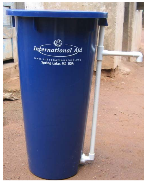
Figure 21: Assembled BioSand Filter ready for installation during Phase 1
