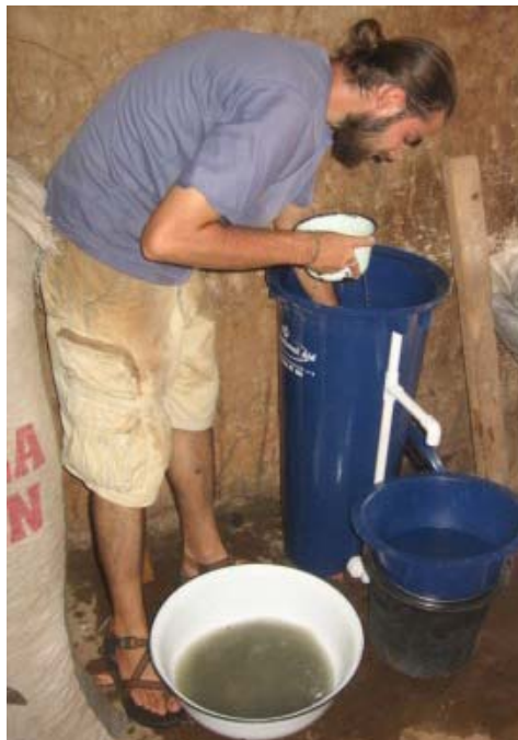
Figure 29: Swirl-and-dump maintenance performed to increase flow rate (Photo courtesy of Carl Allen, 2007)
