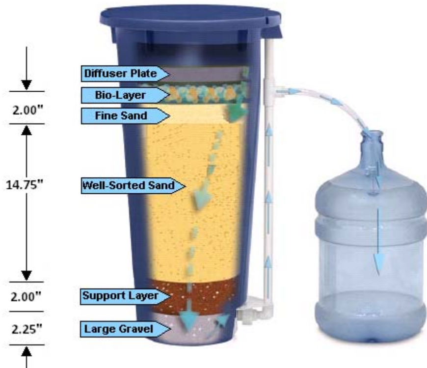
Figure 20: Cross-section of the International Aid HydrAid™ BioSand Filter (Adapted from www.hydraid.org )
