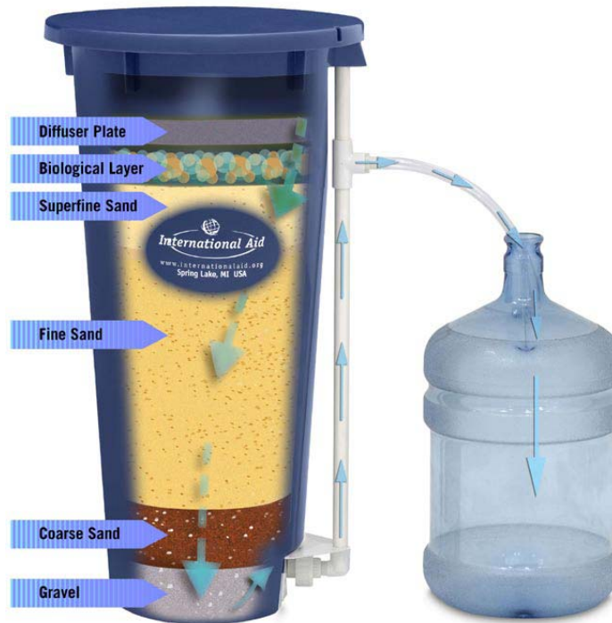
Figure 10: How it Works – HydrAid™ BioSand Water Filter by International Aid ( www.hydrAid.org )
