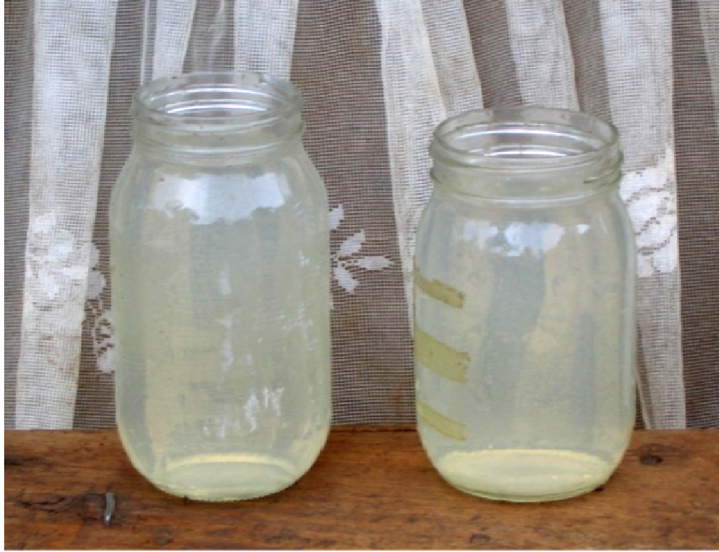
Figure 69: Effluent water sample (right) from HydrAid™ BioSand Filter Sibi 05 showing “No Apparent Change” in color in comparison with the raw source water (left)
