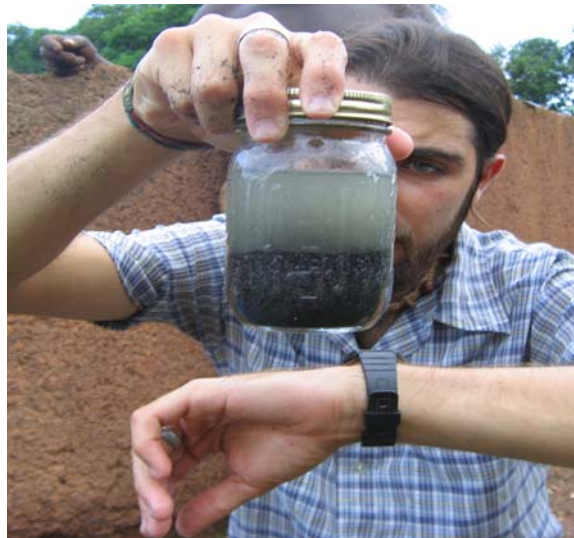
Figure 24: Jar test performed to determine if the sand has been washed thoroughly
