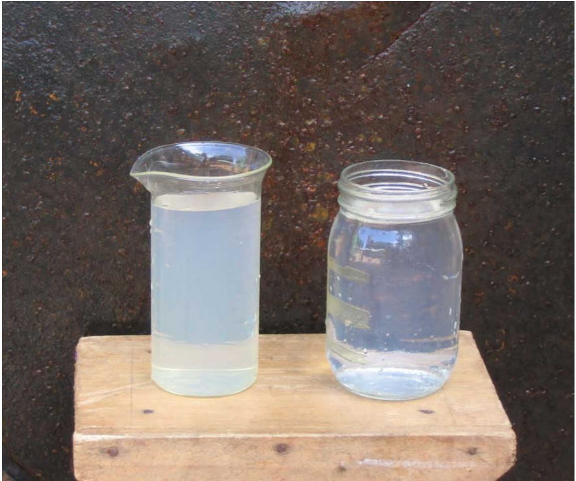
Figure 72: Effluent water sample (right) from HydrAid™ BioSand Filter Sibi 06 showing “Clear” color in comparison with the raw source water (left)
