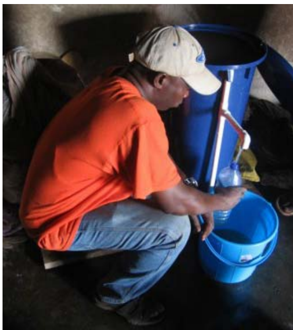
Figure 34: Water sample collection of filtered water from BSFs by re-using 1.5 liter water bottles (Photo courtesy of Carl Allen)
