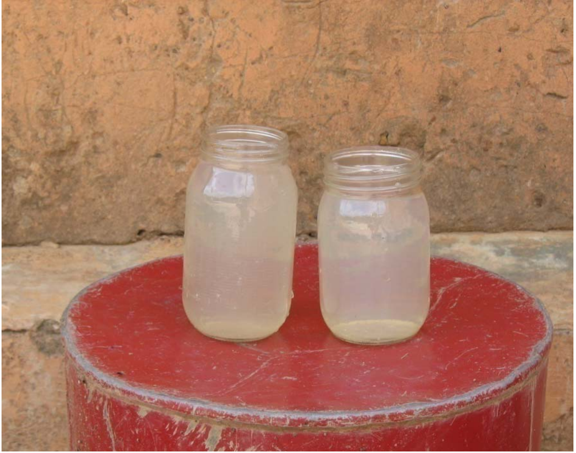
Figure 78: Effluent water sample (right) from HydrAid™ BioSand Filter Sibi 08 showing “Improved” color in comparison with the raw source water (left)
