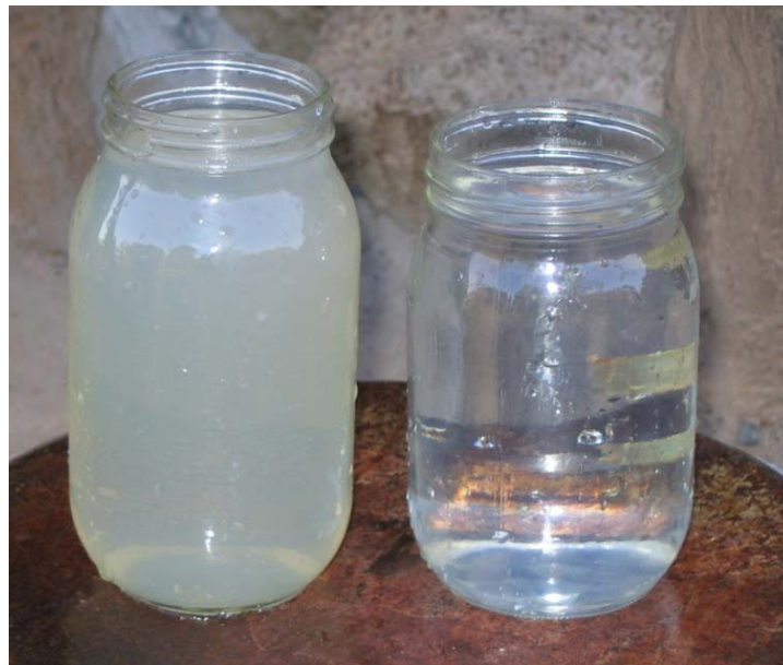
Figure 60: Effluent water sample (right) from HydrAid™ BioSand Filter Sibi 02 showing “Very Clear” color in comparison with the raw source water (left)
