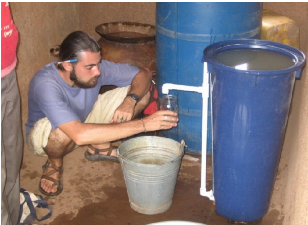
Figure 22: Flow rate measurement test of HydrAid™ BioSand Water Filter (Photo courtesy of Carl Allen, 2007)
