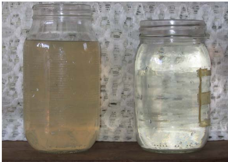
Figure 50: Photograph of the influent (left) and effluent (right) water samples from HydrAid™ BioSand Filter Sibi 03, which shows a clear improvement in color.
