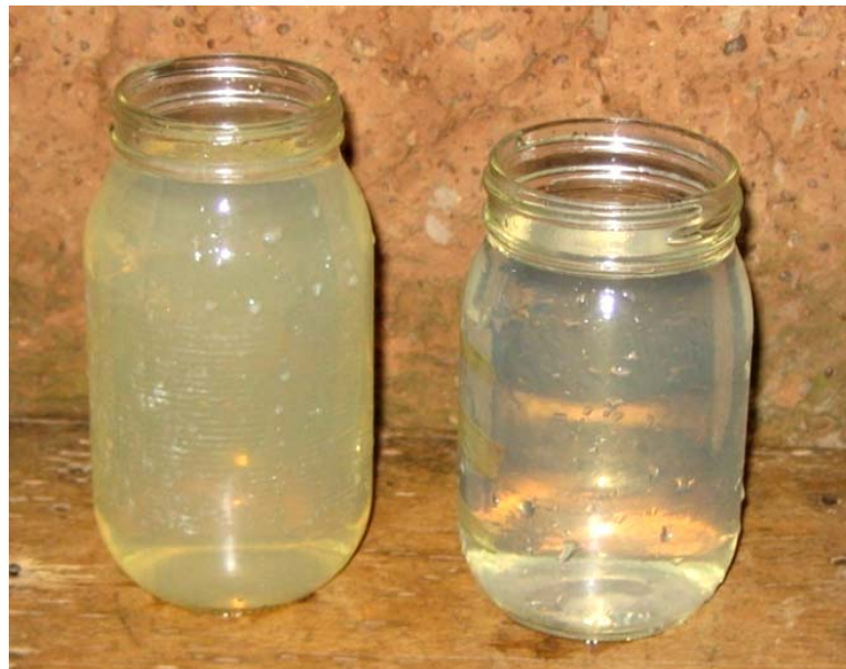
Figure 90: Effluent water sample (right) from HydrAid™ BioSand Filter Sibi 12 showing “Improved” color in comparison with the raw source water (left)
