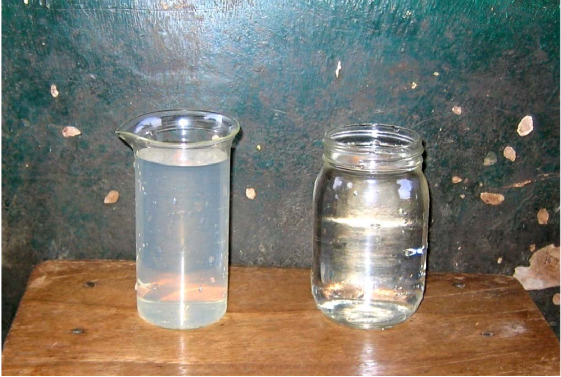
Figure 84: Effluent water sample (right) from HydrAid™ BioSand Filter Sibi 10 showing “Very Clear” color in comparison with the raw source water (left)
