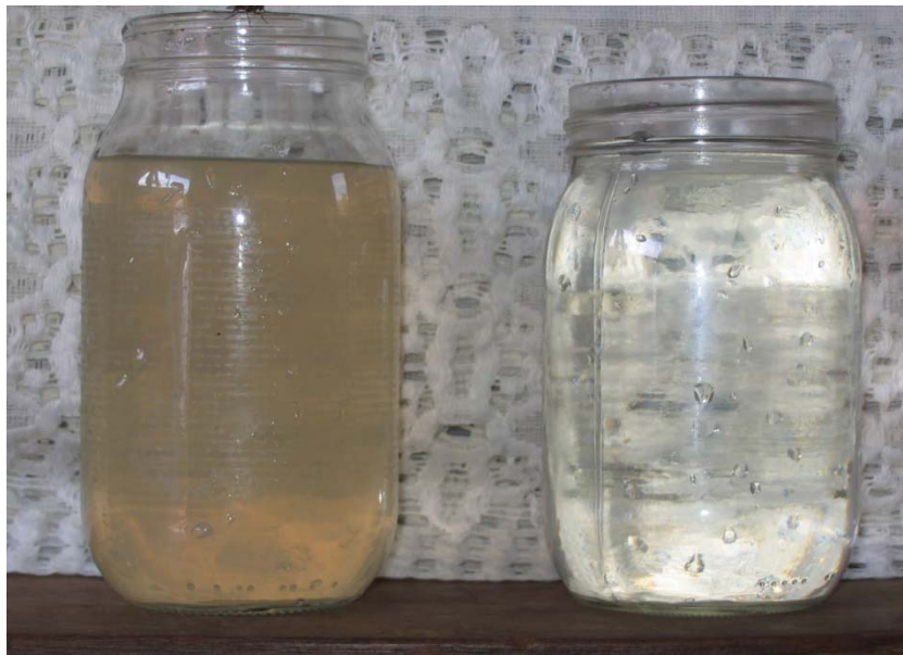
Figure 63: Effluent water sample (right) from HydrAid™ BioSand Filter Sibi 02 showing “Very Clear” color in comparison with the raw source water (left)
