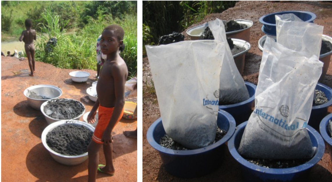
Figure 26: The BioSand filter media after it has been washed and separated (Photos courtesy of Carl Allen, 2007)
