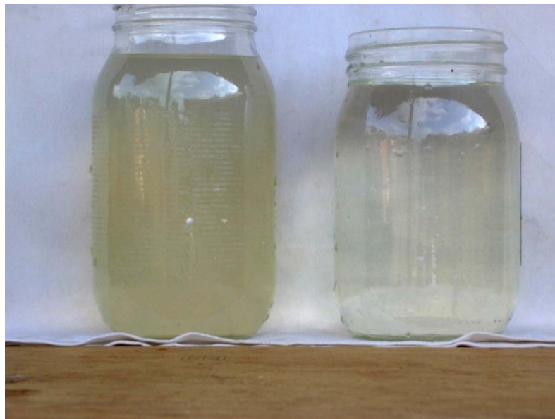
Figure 57: Effluent water sample (right) from HydrAid™ BioSand Filter Sibi 01 showing “Clear” color in comparison with the raw source water (left)
