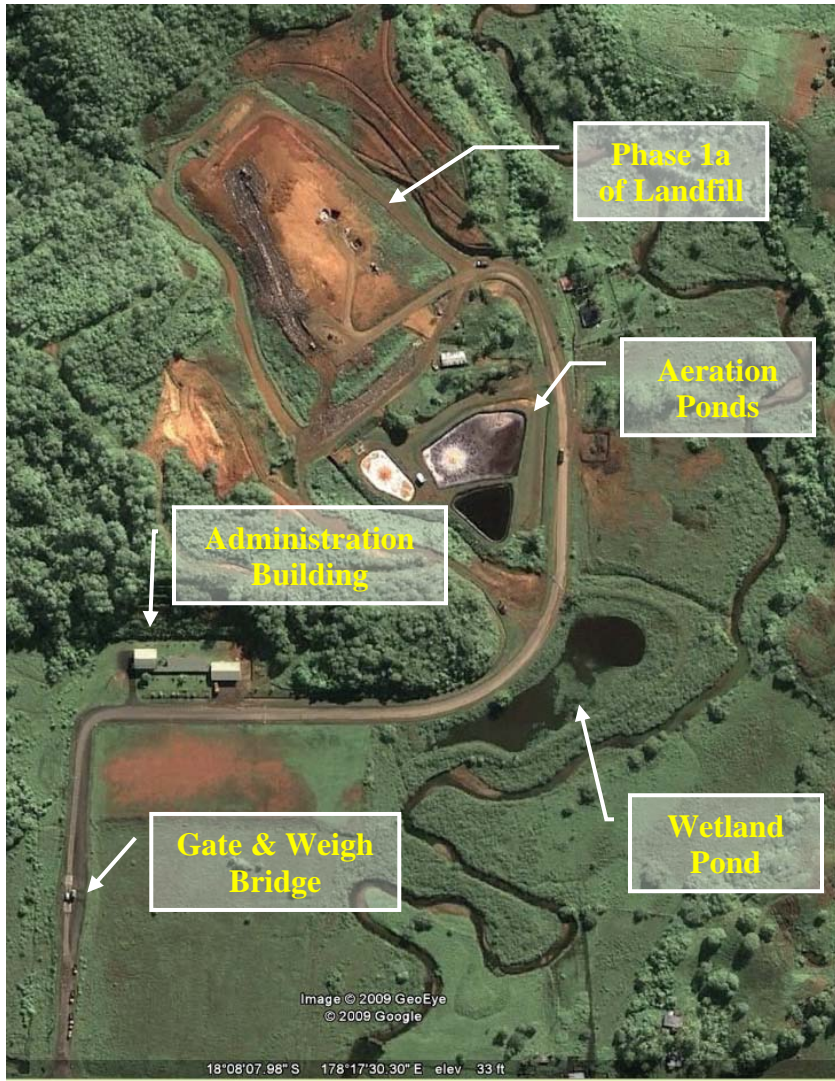
Figure 6: Naboro Landfill compound layout (Google Earth, 2009).
