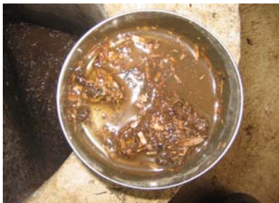
Figure 19: Mixing compost with water to take pH measurement.
