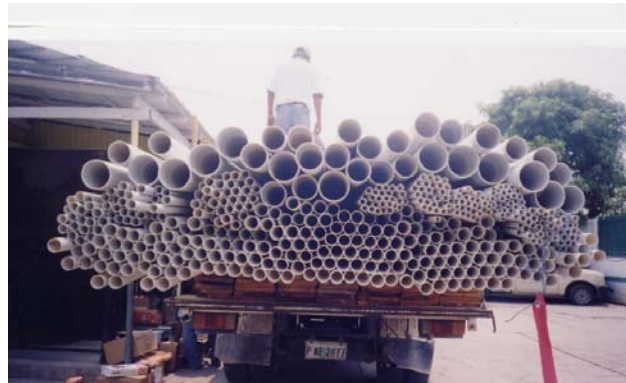
Figure 3-4: Example of various diameter PVC tubing loaded on truck ready for delivery to 2 separate communities. The 3" and 4" tubing is for a community of 150 houses and the 1 ½" and 1" tubing is for a community of 19 houses. The ½" tubing is for both communities for the connections at each house.
