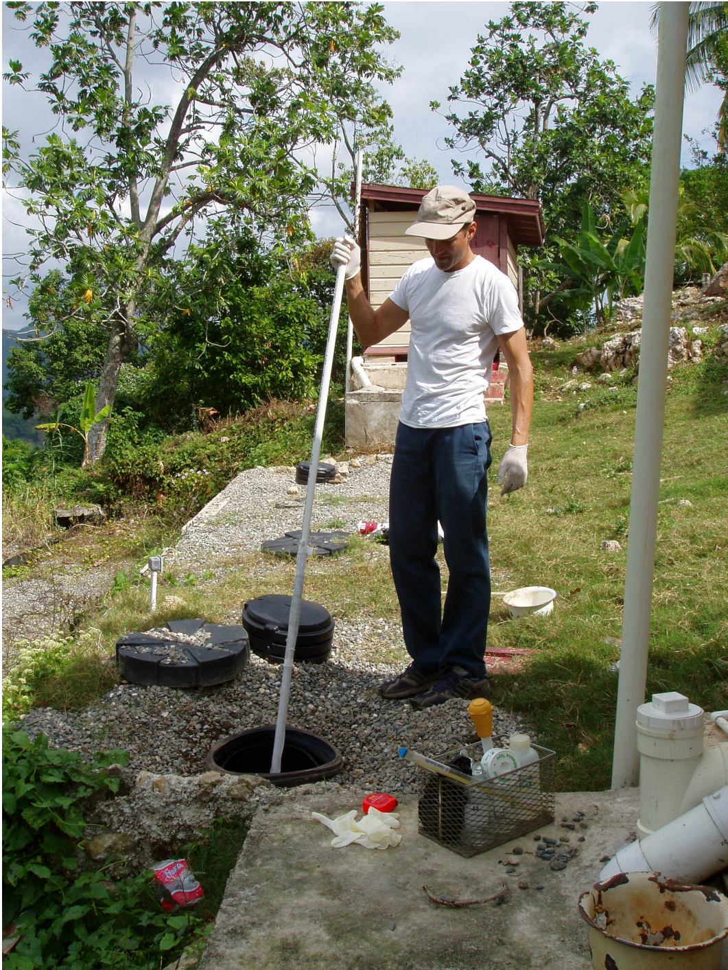
Figure 4-4 Determining septic tank sludge depth using dip stick at Pisgah. (Photograph of author.)
