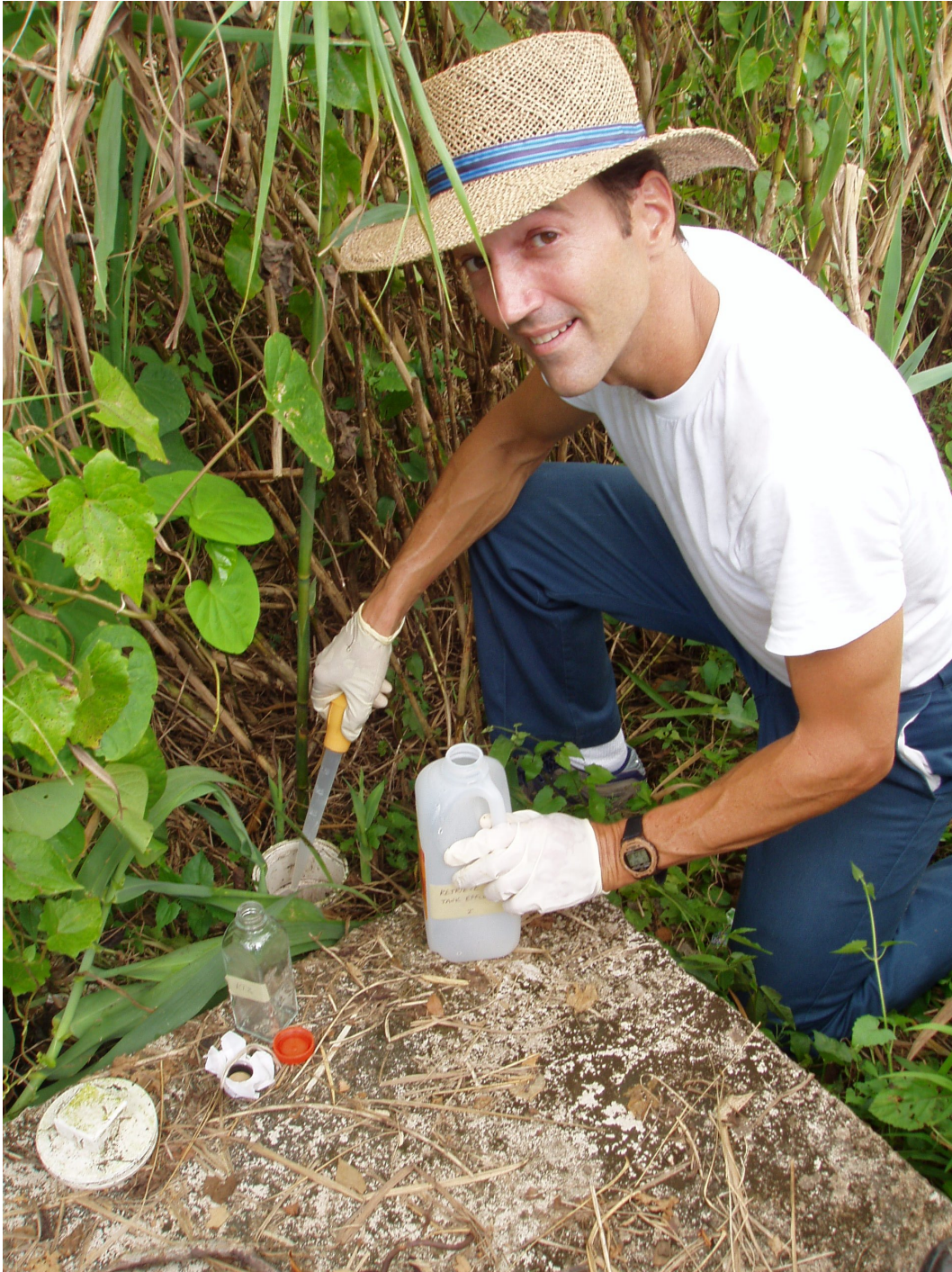
Figure 4-1 An example of grab sample collection. The author is using a syringe to collect the wetland inlet water quality sample at Retrieve. (Photograph of author.)
