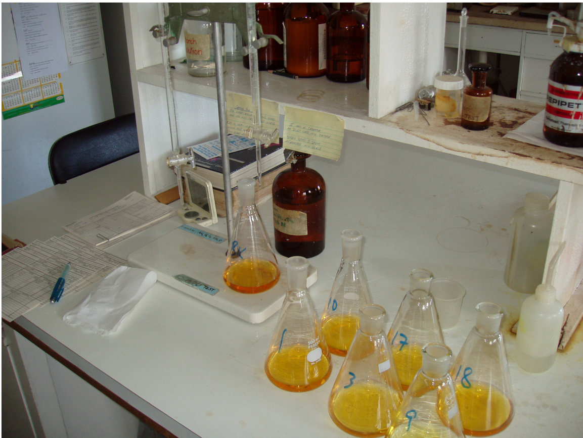
Figure 4-5 Dissolved oxygen titration for BOD test. (Photograph by author.)
