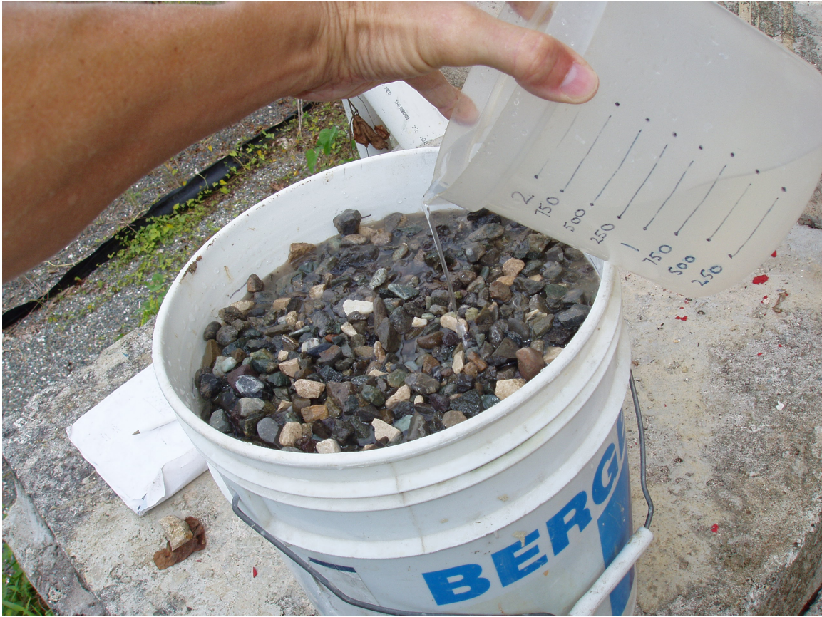
Figure 4-3 Media porosity measurement using a 5-gallon bucket at Pisgah. (Photograph by author.)
