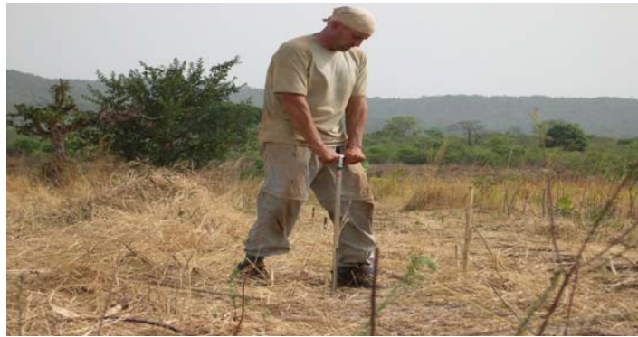
Figure 47 Taking soil samples with soils auger. Photo by Brian Satterlee.
