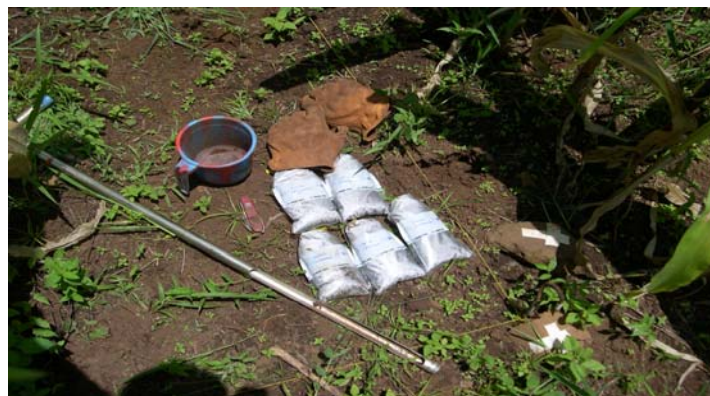
Figure 48 Soils auger and bagged soils samples. Photo by Brian Satterlee.
