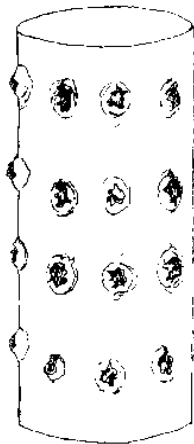
FIG. 15-5. PUNCTURED METAL CASING USED AS WELL SCREEN
