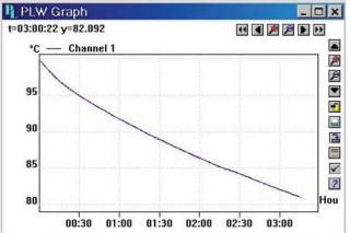
results (results not shown). The insulation is three layers of three-quarter inch thick foam wallboard insulation. There is no inner container and the pot is placed in the open space provided by the layers of insulation. The lack of an inner container allows any spilled foods to get between the insulation layers where it would be hard to clean. While the thermal characteristics are fair, it would not have a very long life in practical field use.
