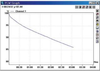
makes up for the extra loss of an inner container. After three hours, the 5 liters of water is above 87°C. This could be expected to produce excellent results. The durability of this RHC structure will withstand extended field use.
