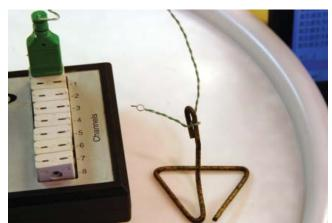
Photo 1 - Thermocouple Support
