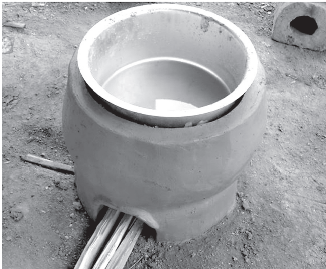
Figure 22: Unfired mud or clay rocket stove. Photo courtesy of Aprovecho Research Center
