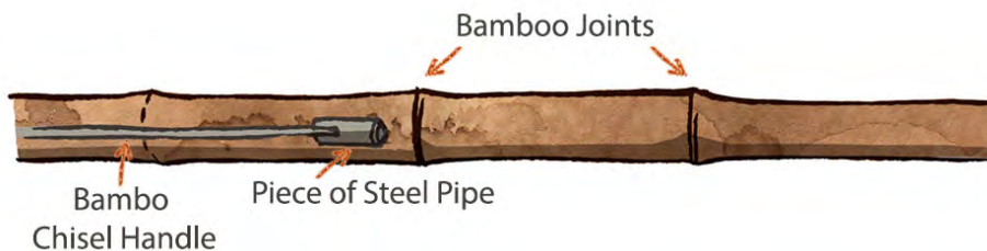
Figure 6-10: Joining Two Pieces of Bamboo
