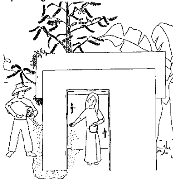
Figure 40: Site Preparation: Spreading Lime
