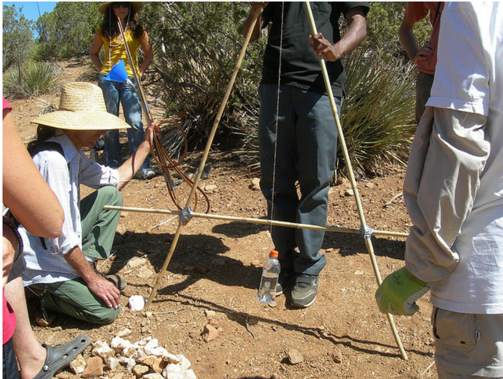
Figure 4-21. Using an A-Frame to Determine Contour Lines
