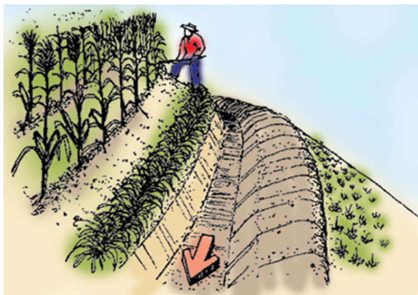
Figure 4-5. Contour Ditches to Catch and Hold Water and Sediment
