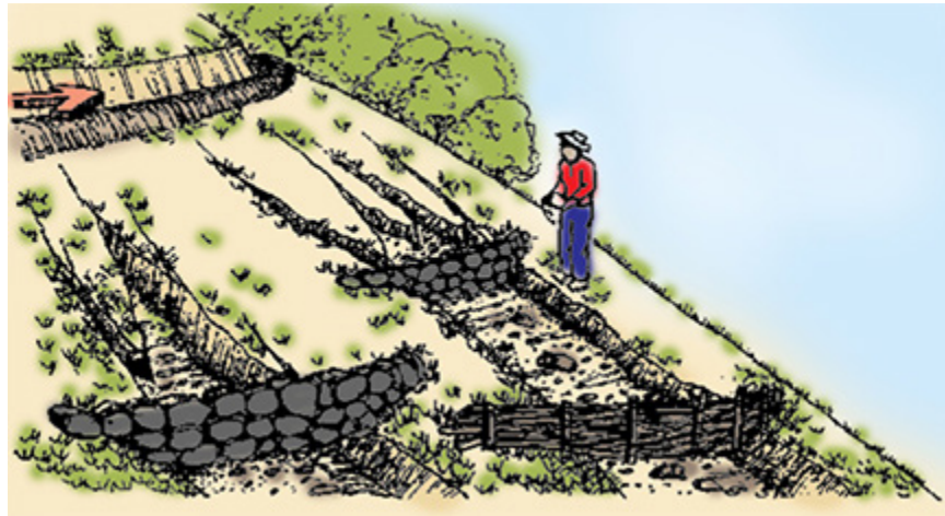
Figure 4-3. Check Dams Made from Rocks or Tree Limbs and Vine
