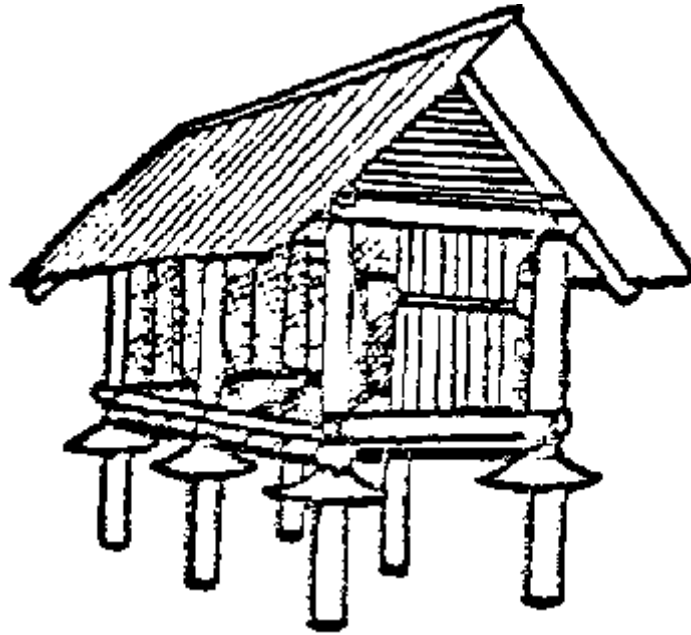
Fig, 53 Improved crib built from imported materials, Swaziland
