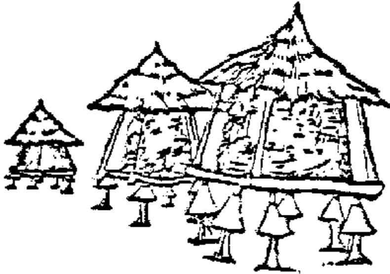
Fig. 51 Improved maize crib built from local materials, Nigeria
