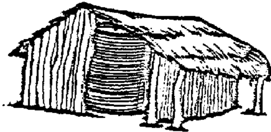
Fig. 58 Imported steel grain silo, Benin
