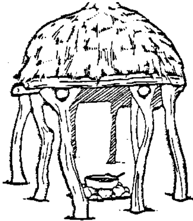
Fig. 8 Improved post-harvest air dryer for rice, Sierra Leo
