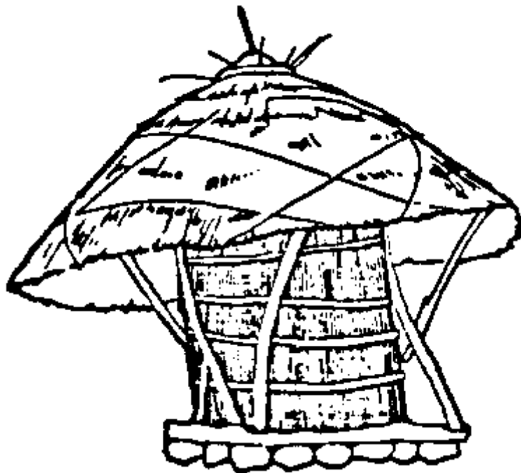
Fig. 33: This store can hold 1,000 kg. of maize on the cob, which is why it is not raised too high off the ground. The door is not protected from birds or rats.
