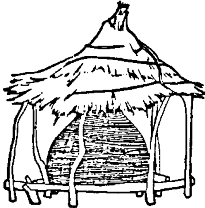
Fig. 32: Similar to Fig. 31, cylindrical basket, raised up on rock footings, with wide, overhanging thatch roof.
