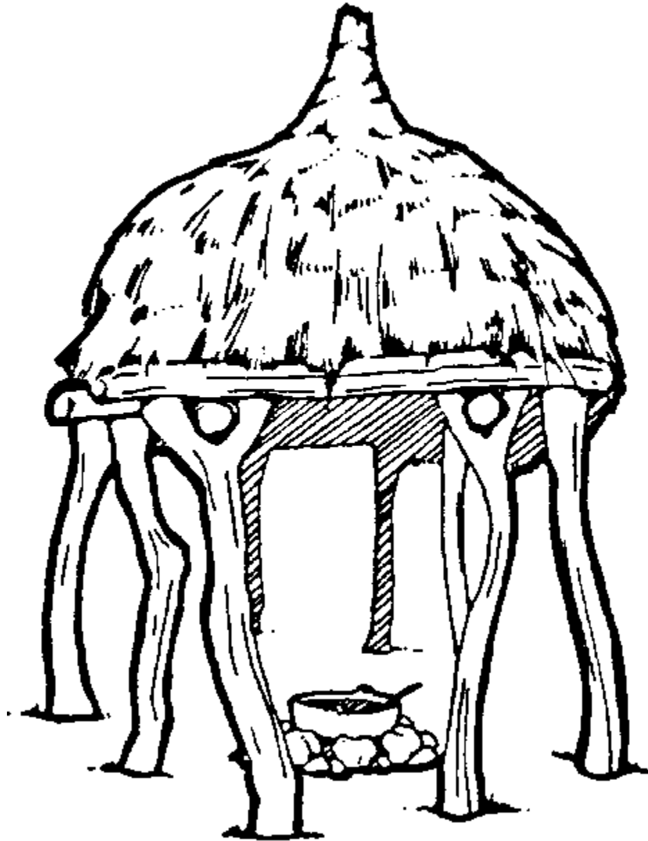
Fig. 8: This air-dryer will hold many "ties" of rice after it is harvested so that the rice does not have to be stacked up in the field where it can easily mold. The device is made from local "bush poles" and can be covered by a thatch roof to keep off rain during the wetseason harvest.
