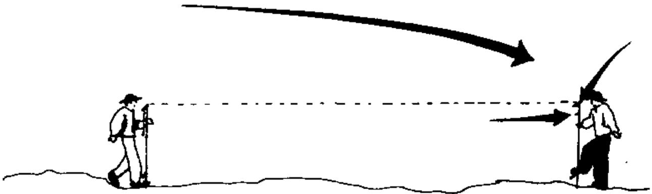
For .5% slope, drain off channel, move sight line 5cm every 10 meters between the two men (up or down depending on which way you want water to run), towards sight man or "maquina" man.
