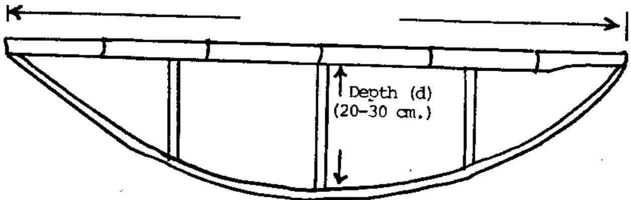
The rear part of terrace, called the toe-drain, functions as a drainage ditch toward the waterway.
