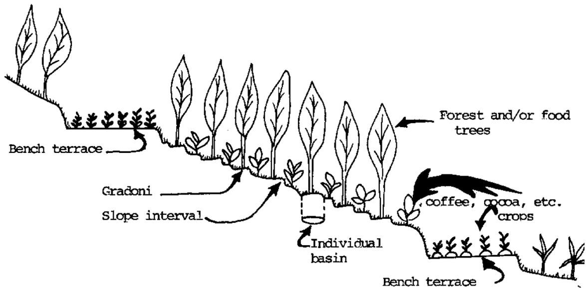
Individual basins can be substituted for the gradonis. Round basins are constructed (about 1m in diameter) with a 10% back slope. The trees are planted in center of the basin.
