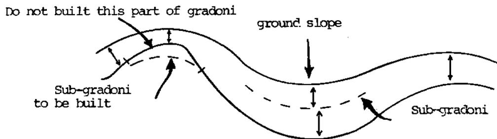
Bench Terraces - Bench terraces are too expensive to construct for forest plantings alone. They are, however, used in agro-forestry projects (EMDEFOR is experimenting with them). Crops are grown on the bench terraces; trees are grown on the slopes between the terraces. For additional soil stabilization, the trees should be planted on gradonis also. This practice affords needed W/S protection while allowing the landowner to farm part of the land. see Fig. 63.
