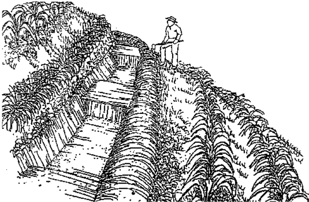
Figure 2.16 Bench Terrace Construction Sequence "A" (Ref. 9)
