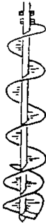
Figure 3.41 Typical Hand Augers and Equipment (Ref. 15) (b) Cohesive Soil Augers
