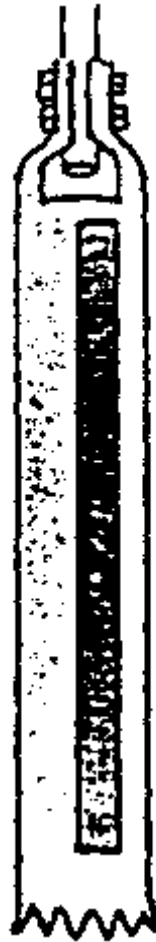
Figure 3.41 Typical Hand Augers and Equipment (Ref. 15) Bucket Auger
