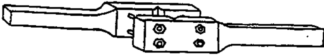
Figure 3.42 Rod or auger Fork Locally Fabricated From 1/4" (6 mm) Steel Plate (Ret. 15)
